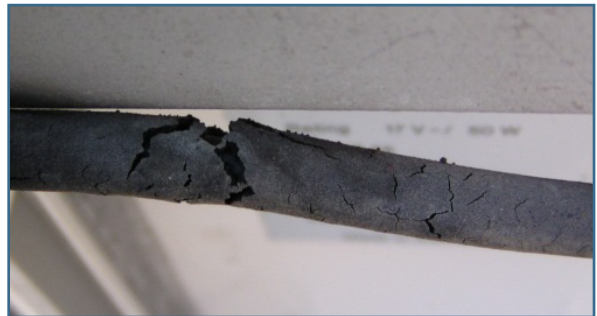
Ozone damage effect
